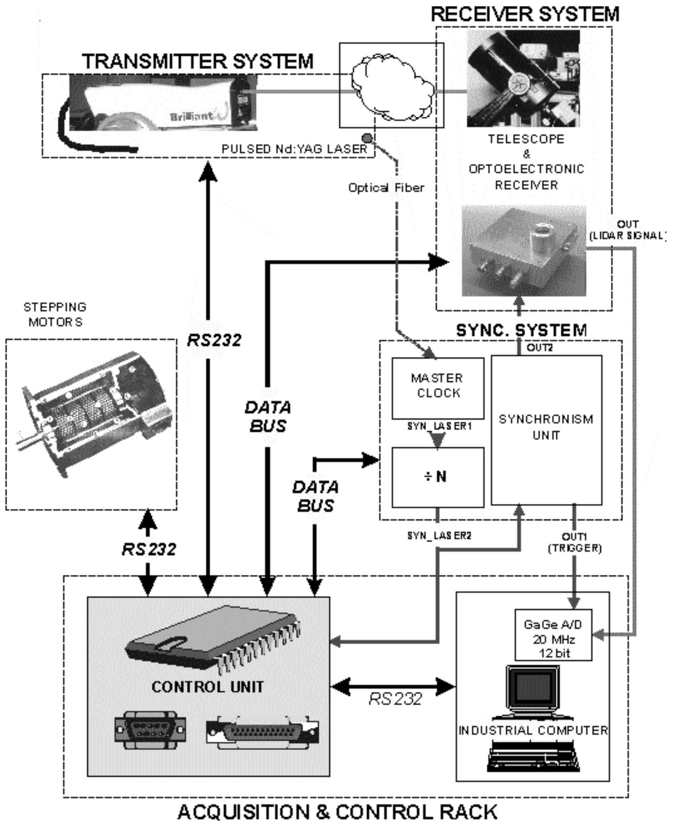
Fig. 3 Lidar system architecture overview showing main units.
