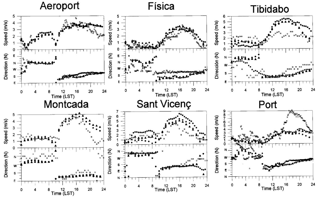
Figure 8. Wind speed and direction calculated by the model for different grids (coarse ●, medium ▲ and fine ◆), compared to surface station measurements □.
