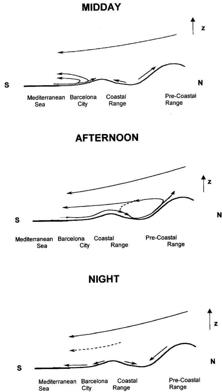
Figure 10. Schematic vertical cross-sections of atmospheric circulations in the Barcelona Air Basin during a typical summer day during midday, afternoon and night periods.
