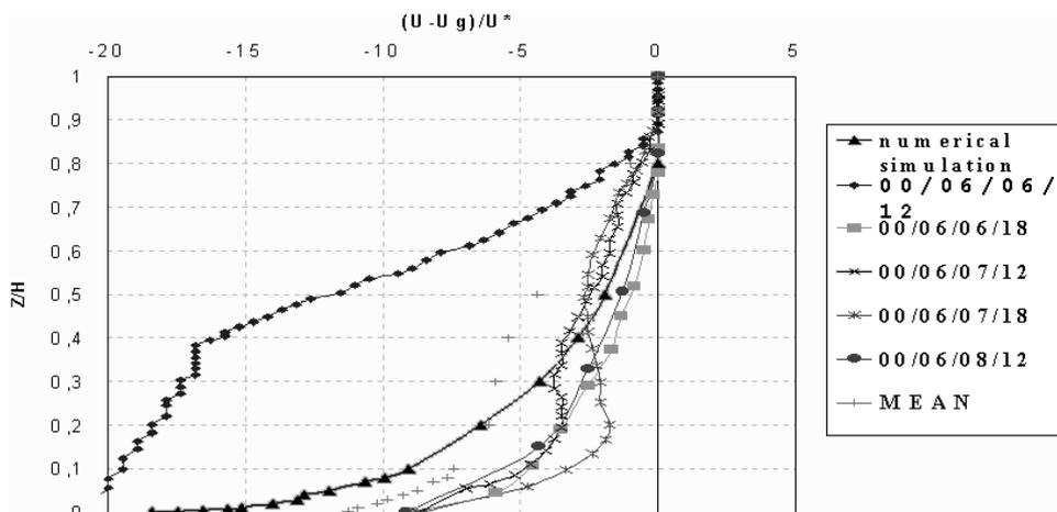
**Figure 8** Comparison of velocity defect profiles inside the UABL simulation with sodar measurement in Prague (Date and time of the observation is in the form yy/mm/dd/hh/mm, W wind direction on the top of the UABL)
