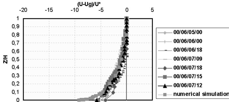
**Figure 7** Comparison of velocity defect profiles inside the UABL simulation with radiosounding launched in Neves Corvo (Date and time of the observation is in the form yy/mm/dd/hh, NW wind direction on the top of the UABL)
