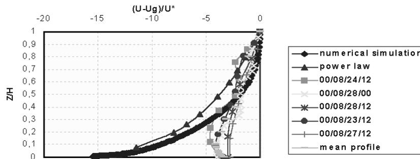
**Figure 6** Comparison of velocity defect profiles inside the UABL simulation with radiosounding launched in Évora (Date and time of the observation is in the form yy/mm/dd/hh, NE wind direction on the top of the UABL)
