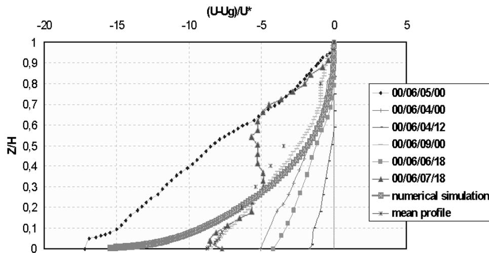
**Figure 5** Comparison of velocity defect profiles inside the UABL simulation with radiosounding launched in Barcelona (Date and time of the observation is in the form yy/mm/dd/hh, SE wind direction on the top of the UABL)
