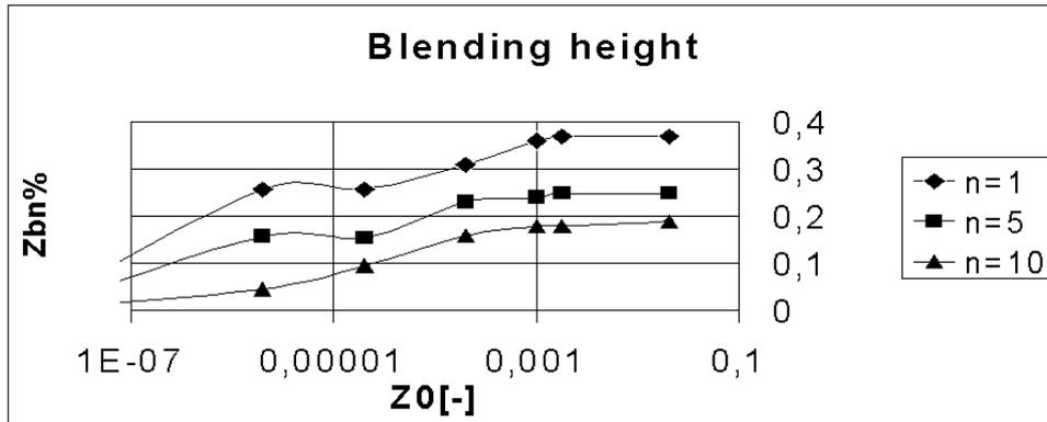
The result can be interpreted that the blending height  $z_b$  (in full scale) for urban area under the simplified assumptions made here with roughness length  $z_0$  more than 1 m is of the order 200 m, i.e. double of the surface boundary layer height – see. e.g. Rotach et al. [5].
