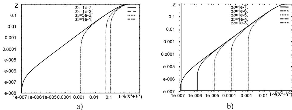
All determined profiles coincide in the upper part, which means that the Rossby number similarity exists there under the very idealized assumptions made here. The profiles are splitted in the lower part – the Rossby number similarity is not existent. It can be assessed that the height  $Z_b$ , where the Rossby number similarity exists, is roughly
